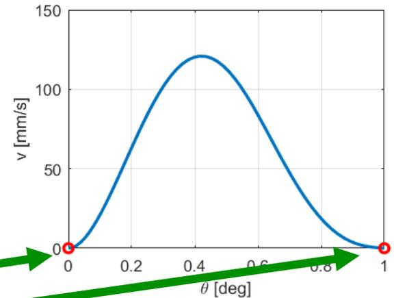
$$\begin{aligned} s'(x_0) &= 0 \\ s'(x_3) &= 0 \\ s''(x_0) &= 0 \\ s'''(x_3) &= 0 \end{aligned}$$
